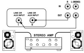
To connect the monitor to stereo system speakers:
